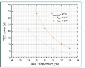
Power consumption of the built-in TEC¹ as a function of the QCL chip temperature for a base plate temperature of +40°C, with and without a thermal load in the QCL.
