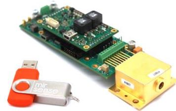
**PowerMir** product line is high power pulsed Quantum Cascade Laser based on proprietary technology, emitting in Mid-Infra-Red. It provides maximum average power of minimum 1 Watt at 4 microns. This system is made up of a QCL HHL-packed laser plugged to an OEM PCB board. Onboard software and Windows software are both provided.
