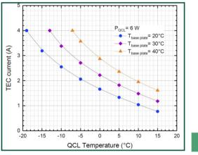
TEC current consumption as a function of the wanted QCL chip temperature for different base plate temperatures and for a QCL thermal load of 6 W.
