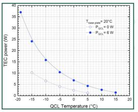
Power consumption of the built-in TEC¹ as a function of the QCL chip temperature for a base plate temperature of +20°C, with and without a thermal load in the QCL.
