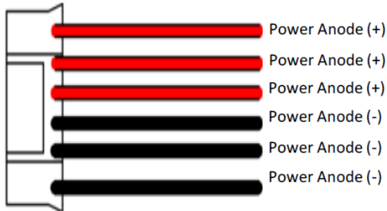
Connection of Power Supply Line (6 PIN)
