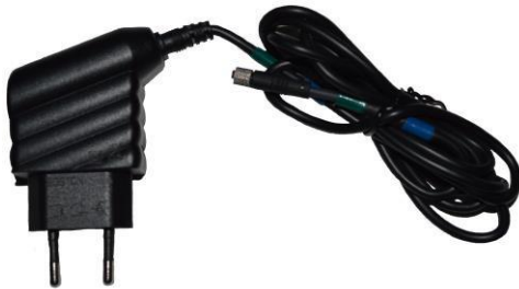
Wall-plug Power Supply for 12V DC Laser Diode Module.
