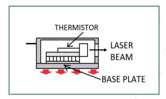
The above HHL-package diagram shows the built-in thermistor that monitors the laser chip temperature. The diagram also shows the base plate that dissipates the heat generated by the TEC and the laser chip.
