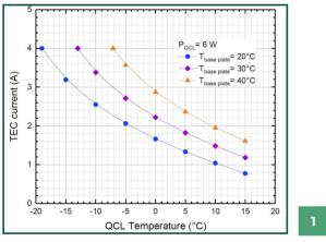
TEC current consumption as a function of the wanted QCL chip temperature for different base plate temperatures and for a QCL thermal load of 6 W.
