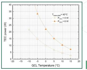
Power consumption of the built-in TEC<sup>1</sup> as a function of the QCL chip temperature for a base plate temperature of +40°C, with and without a thermal load in the QCL.
