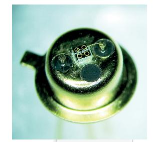
Parallel connection of several LED chips that emit at the same wavelength and driving them together can provide significant increase of total optical power. FLC offers a 4-element LED matrix with one peak wavelength at 3.4 µm or 4.3 µm.
