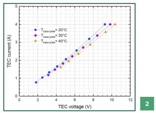
Current-voltage characteristics of the built-in TEC for different temperatures of the base plate.
