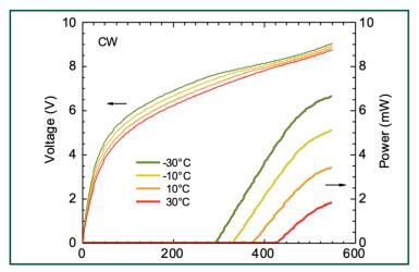
Single Mode Distributed Feedback Quantum Cascade laser at ~746 cm-1
