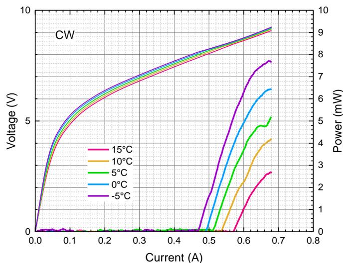
*The curves on the left indicate the voltage of the laser as a function of the applied DC current and laser chip temperature.*
