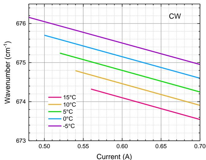
The curves indicate the typical laser singlemode emission wavelength as a function of the applied DC current and laser chip temperature. Lasers with slightly shifted wavelength are also available.
