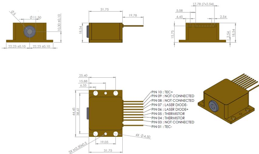
**Electrical connections (pinout MPL):**
