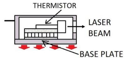
The above HHL-package diagram shows the built-in thermistor that indicates the laser chip temperature. The diagram also shows the base plate that dissipates the heat (because typically the built-in TEC will cool down the laser chip).
